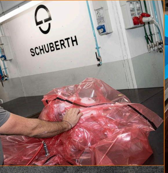
SP1 Carbon is an exclusive autoclave moulded Carbon Fiber shell masterfully handcrafted to give back a unique helmet able to combine lightness, solidness, safeness in an exclusive and iconic design.
