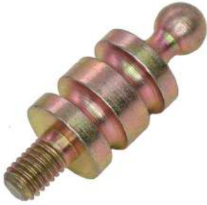
1/4" BALL STUD 22-111 THREADS: 10-32, LENGTH: 1.260"
