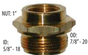
NUT: 1" OD: 7/8" - 20 ID: 5/8" - 18 FUEL FITTING INLET - (OE Style) 90-178
