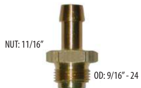
NUT: 11/16" OD: 9/16" - 24 5/16" FUEL INLET FITTING HOSE 90-176
