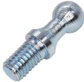
1/4" BALL STUD 22-121 THREADS: 10-32, LENGTH: .750"
