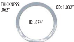
THICKNESS: .062" OD: 1.032" FUEL FITTING GASKET G1126 TEFLON
