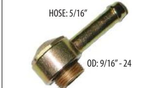
NUT: 11/16" OD: 9/16" - 24 3/8" FUEL INLET FITTING HOSE 90-175
