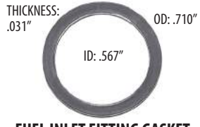
THICKNESS: .031" OD: .710" ID: .567" FUEL INLET FITTING GASKET G1206 RUBBER COATED ALUMINUM
