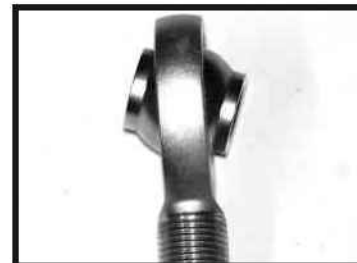
Examine the rod end in this photo closely. See how the ball isn't centered? This is essentially the "misalignment" that the rod end design can handle.
