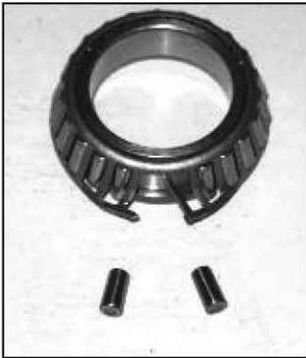
This is a cut-apart view of a tapered roller bearing commonly used as a car type wheel bearing. Notice the inner race where the rollers ride and you can see that it needs to be perfectly smooth. Also of note is the metal cage that holds the rollers together and separates them. This also helps to make the bearing free, with less drag.
