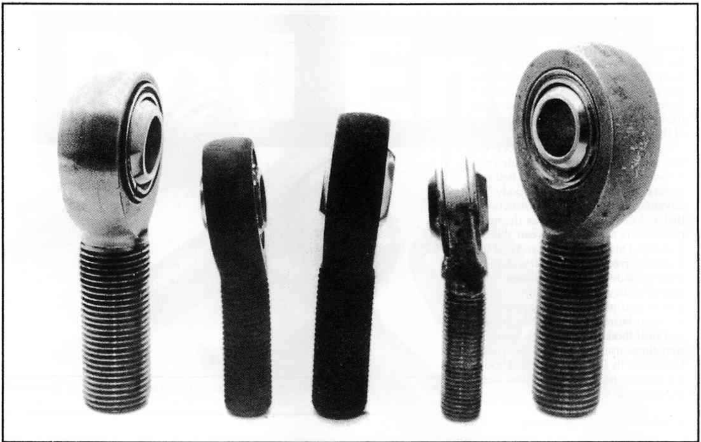
Damaged rod ends. Note insert on far left rod end is partially pushed out. Unit on far right shows dent in race from severe misalignment. Don't do anything with these rod ends except throw them out!
