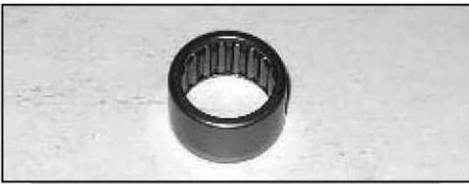
An example of a caged needle bearing. This particular bearing is used as a pilot bearing for a clutch assembly. It is used to keep the transmission input shaft spinning free in the end of the crankshaft. It is a radial load type bearing.
