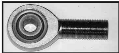
This is a close up look at a heavy-duty rod end. The oversize rod end is generally made by installing an insert one size smaller in the body of the part with the larger shank.
