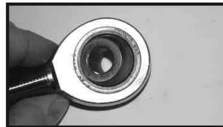
Examine the rod end in this photo closely. See how the ball isn't centered? This is essentially the "misalignment" that the rod end design can handle.
