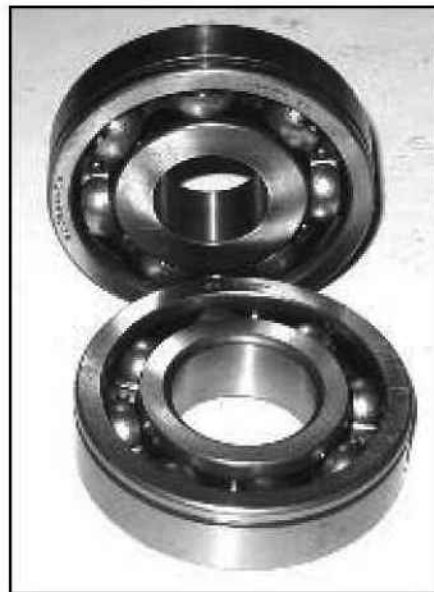
These two bearings are heavy duty ball bearings used for the input and output shafts of a manual transmission. The inner race, the balls, the cage and the outer race are all made together as to ensure maximum load and minimum friction.
