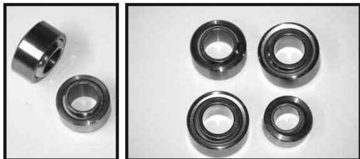
Spherical bearings are actually close relatives of rod ends. They have countless uses in cars. They're often used on custom suspension components - particularly when composite materials are used for construction. Spherical bearings are available in a wide array of bore sizes, usually ranging from 0.1900 to 1.00-inch. In the case of quality components, they're manufactured under the same quality as military approved bearings.
